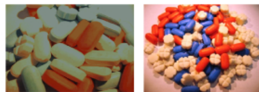
Figure 3—Dry powder ibuprofen tablets film coated using formulations containing (a) Acryl-eze MP or (b) Eudragit EPO.
