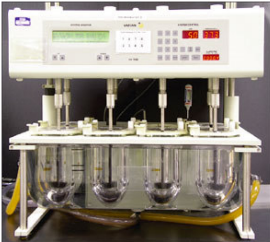
Figure 1. USP Apparatus 2 is generally the first choice for measuring the dissolution of immediate release dosage forms.
