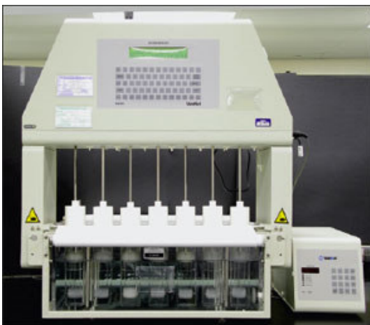
Figure 2. The advantages of USP Apparatus 3 include ease of setup, operation, and sampling. It is generally preferred when a pH gradient is required.
